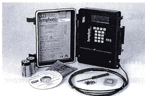
Figure 8: Data Logger, NRG Symphonie Logger (NRG-Systems, 2009)
