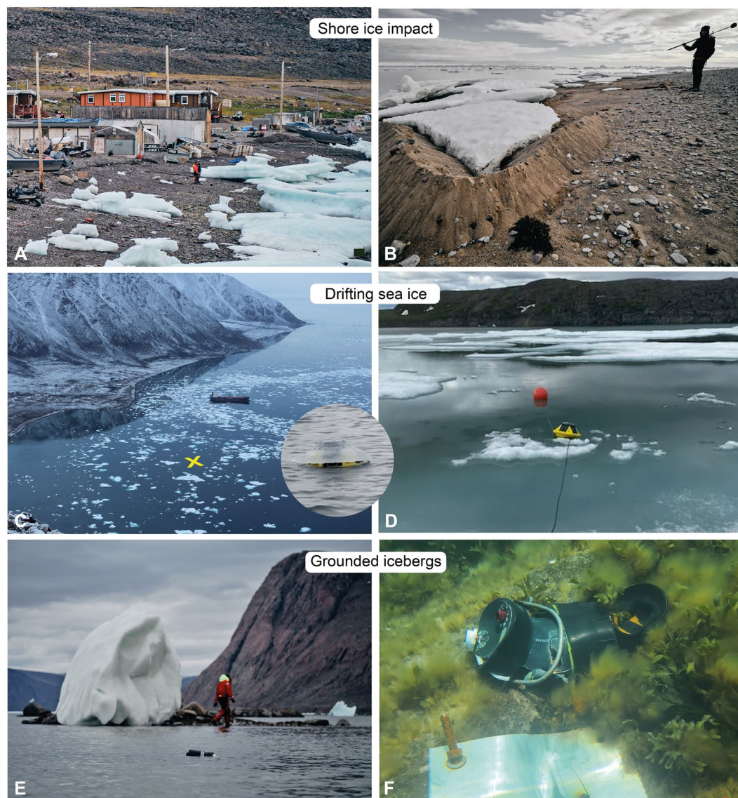
Fig. 11 Sea ice makes wave and water-level observations difficult. (A,B) Shore-fast ice can be grounded on the beach and directly impact sensors that are anchored in shallow areas. (B,C) Drifting sea ice causes the buoys to drift away, and cold air temperatures induce the formation of a thick layer of ice on the buoy's top solar panel. The Ausuittuq buoy is indicated by the yellow x in panel D. (D,E) Grounded icebergs can destroy moored sensors down to several metres depth.
