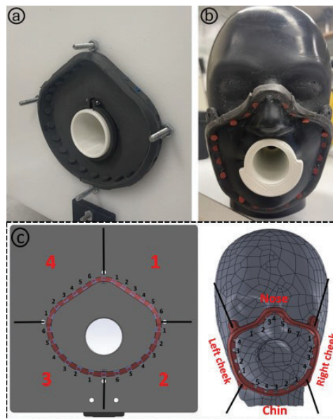
Fig. 4. Control of Number, Size and Location Leak(s)
