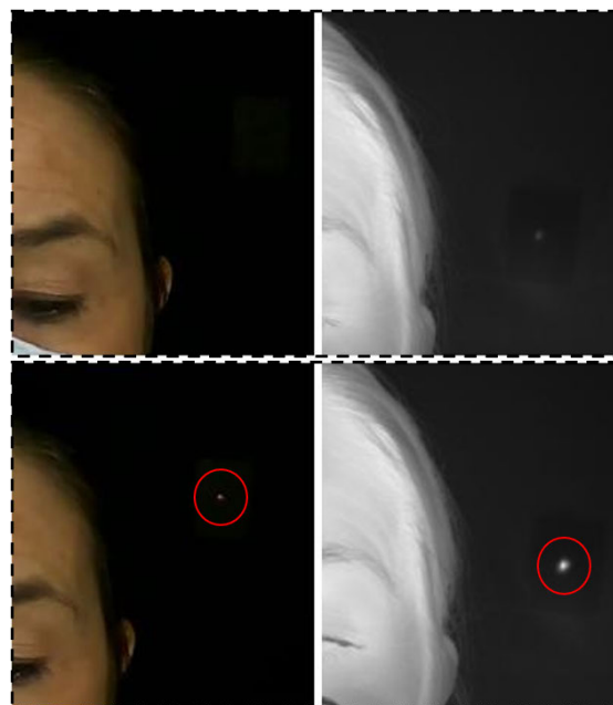
FIGURE 3. Two IR and RGB image pairs with and without pulse of heat and light (encircled in red) for synchronization.
