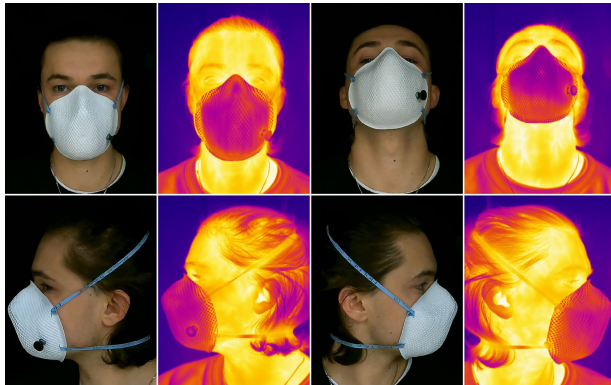
FIGURE 7. Visualization of IR and RGB images in 4 different positions: front, top, left, right.
