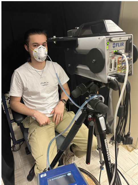
FIGURE 4. Final installation including the imaging system, the PortaCount®, the dark tent and the swivel chair.
