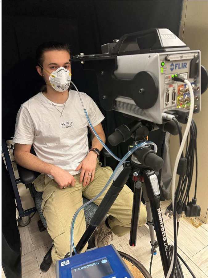
Figure 3.4 Final installation including the imaging system, the PortaCount ® , the dark tent and the swivel chair
