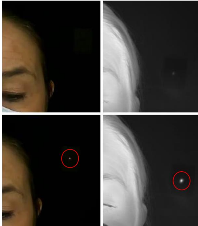
Figure 3.3 Two IR and RGB image pairs with and without pulse of heat and light (encircled in red) for synchronization
