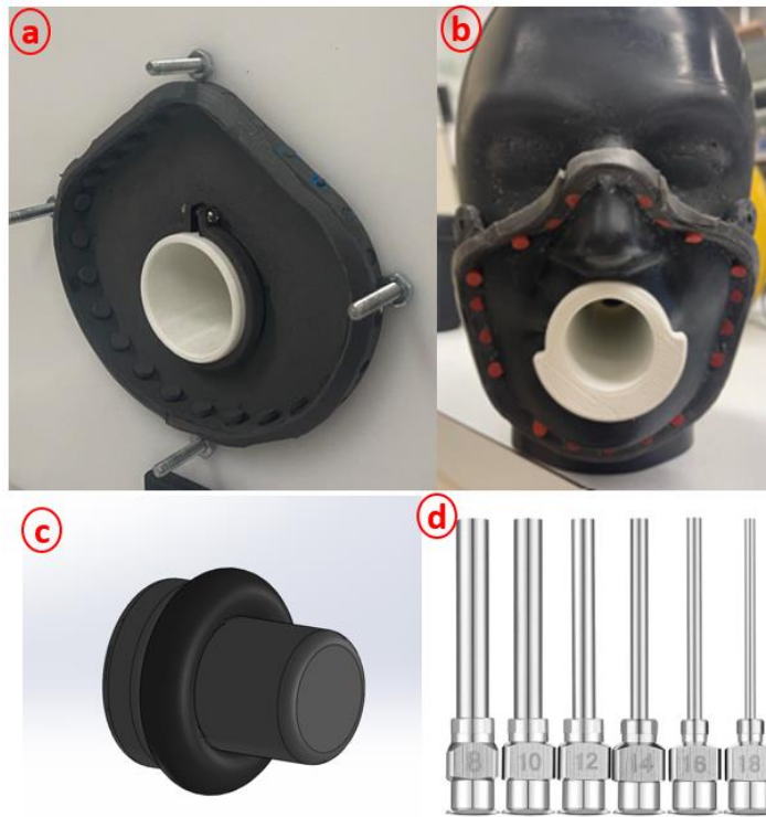
Figure 1.4 Control of number, size and location leak(s)
