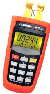
Figure 37 : Thermocouple HH802 Omega (type Alumnel - Chromel)
