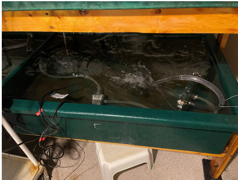
Figure 5. Photo of an acrylic respirometry chamber in the ambient 300 L water bath.
