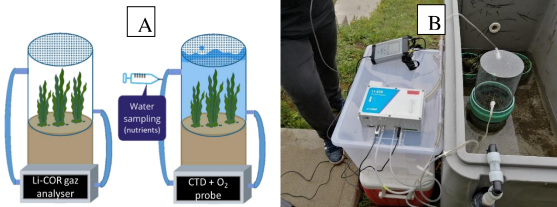
Figure 12 : Incubation set-ups. A : at emersion (left), plugged on an infrared CO 2 gas analyzer, and at immersion (right), plugged on a CTD equipped with an O 2 sensor. Output and input are placed, respectively, at the top and bottom of the cylindrical chamber (V= 9,89 L, d = 20.32 cm, h = 30.4 cm). At immersion, water sampling was made on the output pipe; B : picture of the set-up at emersion. The output pipe was connected to two drying columns avoiding water condensation in the gas analyzer.
