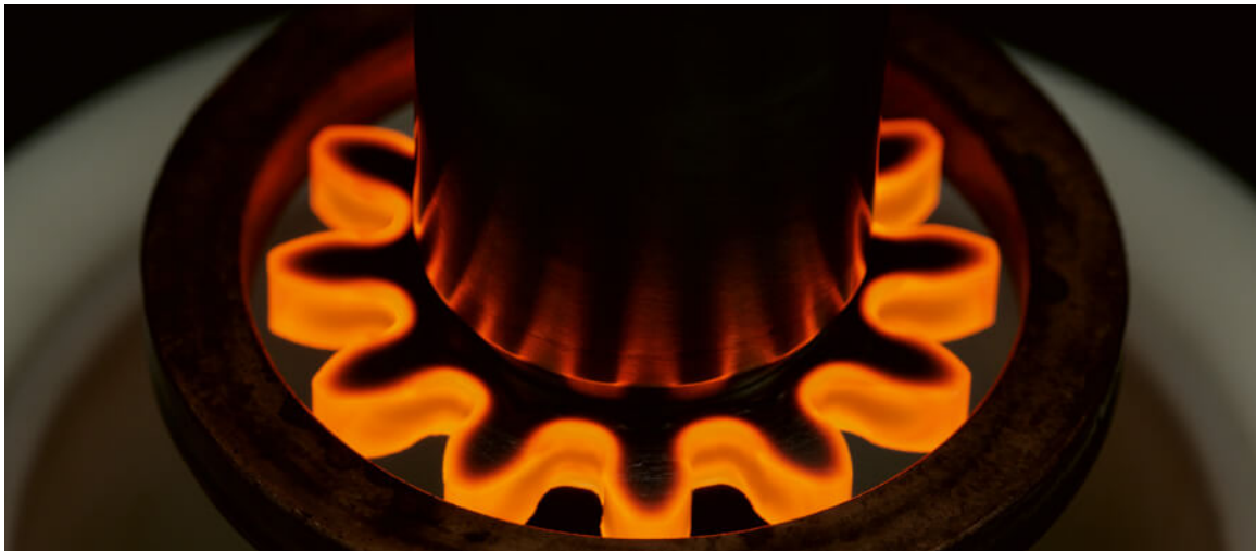
Figure 1.2.6 : Induction hardening of a gear by rotation relative to the inductor
