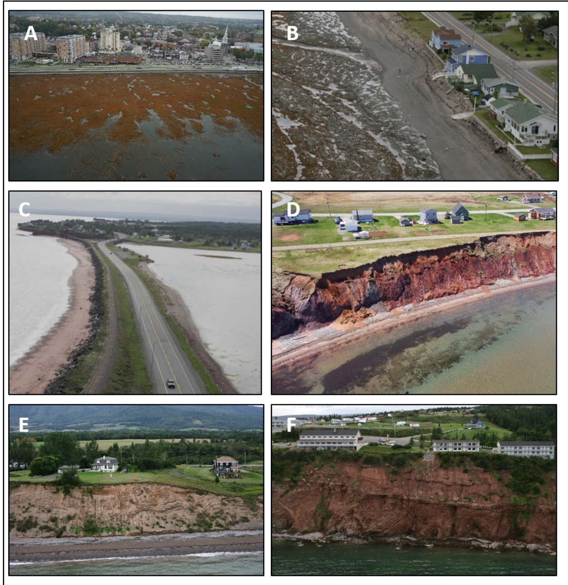
Figure 9. Types of coasts for the Bas-Saint-Laurent and Gaspésie-Magdalen Island regions. (A) Boulevard, hotels and commercial buildings protected by wall in front of a marsh – Rimouski. (B) Houses and national road 132 build on the beach terrace – citizens have put up wall and rock armour, Sainte-Flavie. (C) Railway and national road 132 build on spit protected by rock armour (D) Argillite and glaciomarine cliff – With the cliff retreating, the street was abandoned and two residences were moved, Magdalen Island. (E) Houses on the top of a Sandy cliff, Carleton (F) Motels on the top of a sandstone cliff, Percé
