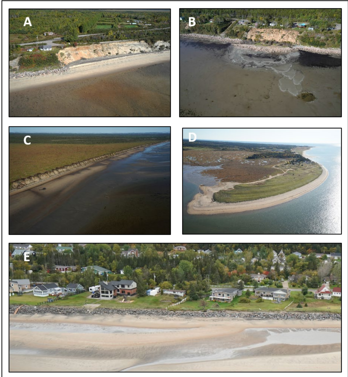
Figure 8. Types of coast on the North Shore of the St.Lawrence river in 2017. (A) Sandy cliff – Rock armour at the left, Pointe-aux-Outardes. (B) Landslide in unconsolidated cliff – The rock armour has been displaced by landslide, Pointe-Lebel. (C) Natural cliff composed of sand, silt and clay, typical of the large deltaic complexes of the North Shore, Pessamit. (D) Spit and marsh, Pointe-à-Boisvert. (E) Beach terrace - Houses protected by Rock armour, Sept-Îles
