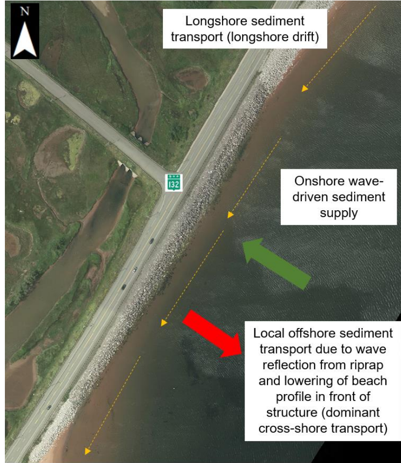
Figure 35: Simplified coastal processes model along the Hope Town coast protected by the riprap (Zone 4).
