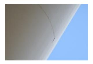
Figure 31. Long leading-edge chordwise crack with spanwise cracking [131]
