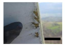
Figure 27. A small area of coating damage [131]
