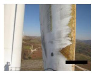
Figure 30. Leading-edge erosion with large exposed surfaces of fiberglass [131]
