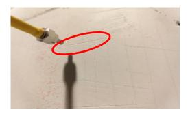
Figure 78. Minor crack on the blade specimen
