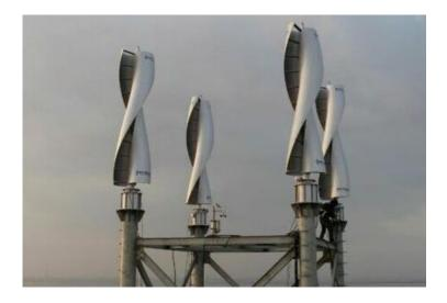
Figure 20. Twisted Savonius turbines
