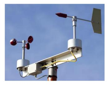
Figure 46. Anemometer and Vane [225]
