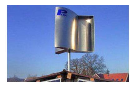
Figure 19. Savonius turbine
