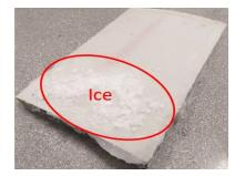
Figure 82. Ice on the specimen
