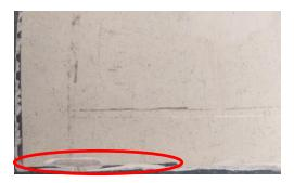
Figure 81. Severe crack on the blade specimen
