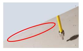
Figure 79. Light erosion on the blade specimen
