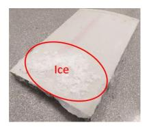
Figure 95. Ice on specimen
