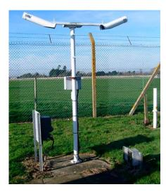
Figure 48. Visibility and Cloud Base Detector [231]
