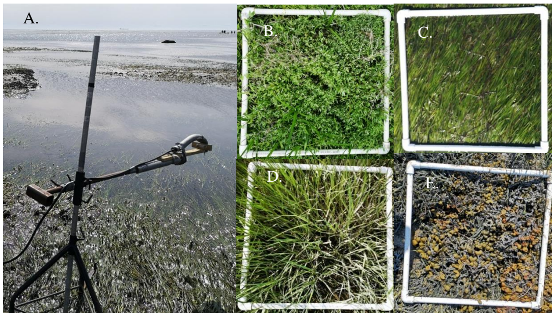
Figure 9. Acquisition of the emerge surface reflectance with the ASD (A.) and the vegetation target such as CS (B.), EG (C.), SC (D.), and MA (E.).
