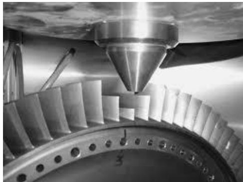
Figure 1. 4. The repair of damaged Titanium blisk using lasers metal deposition process [29].
