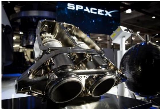
Figure 1. 2. SpaceX AM built Super Draco rocket engines [24].
