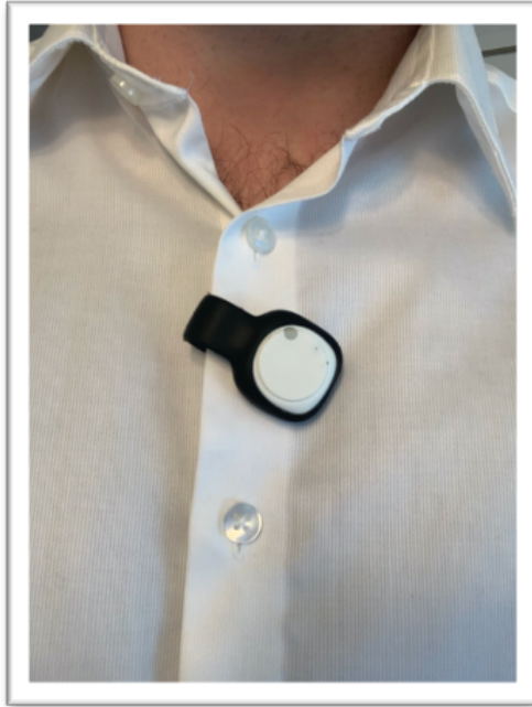
Figure 10: MetaMotionC (MMC) placed on the chest.
