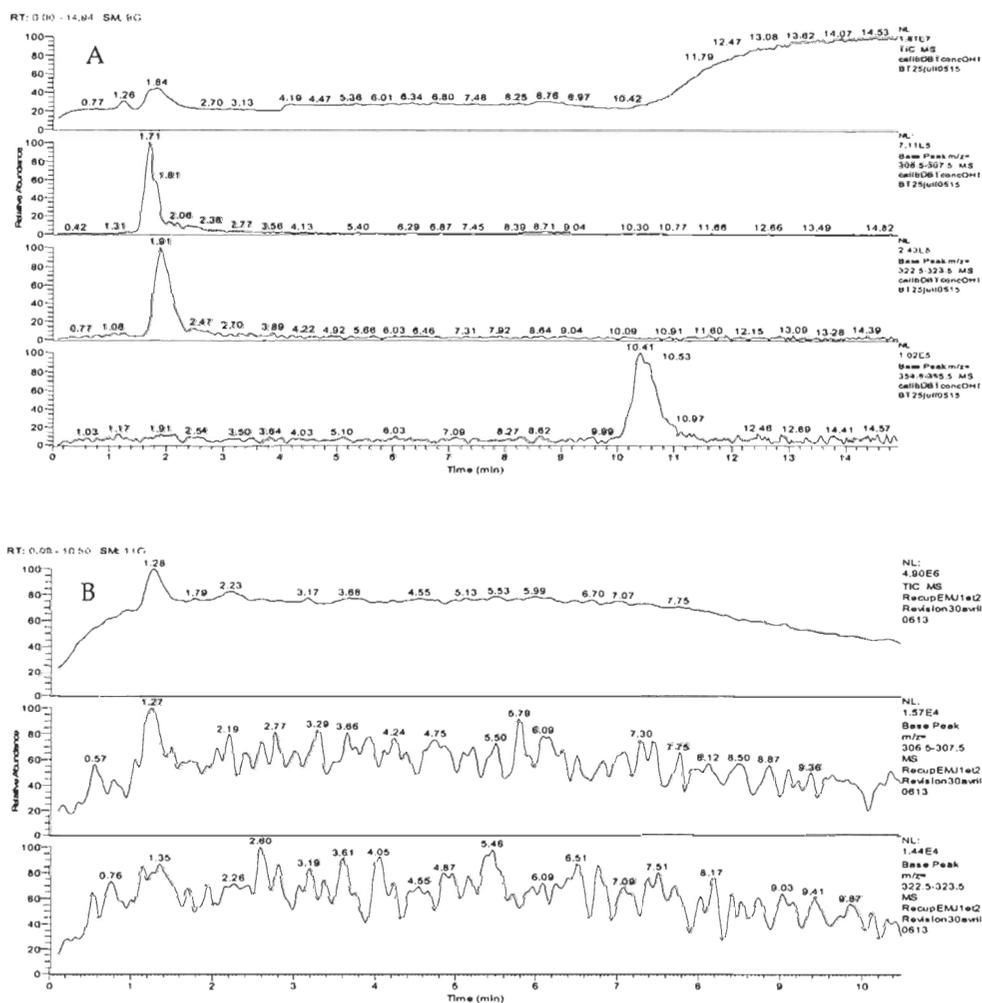
Fig. 3. Typical LC-APCI-MS chromatograms for (A) butyltin standard ( $2 \mu\text{g mL}^{-1}$ ) using a Discovery® Cyano column: OHBuDBT (RT= 1.71 min); TBT (RT = 1.91 min) and DBT (RT = 10.41 min); (B) analytical blank extract, and (C) a sample of seawater spiked at  $0.4 \mu\text{g mL}^{-1}$  of both analytes (RT= 3.31 min for OHBuDBT and RT = 3.96 min for TBT).
