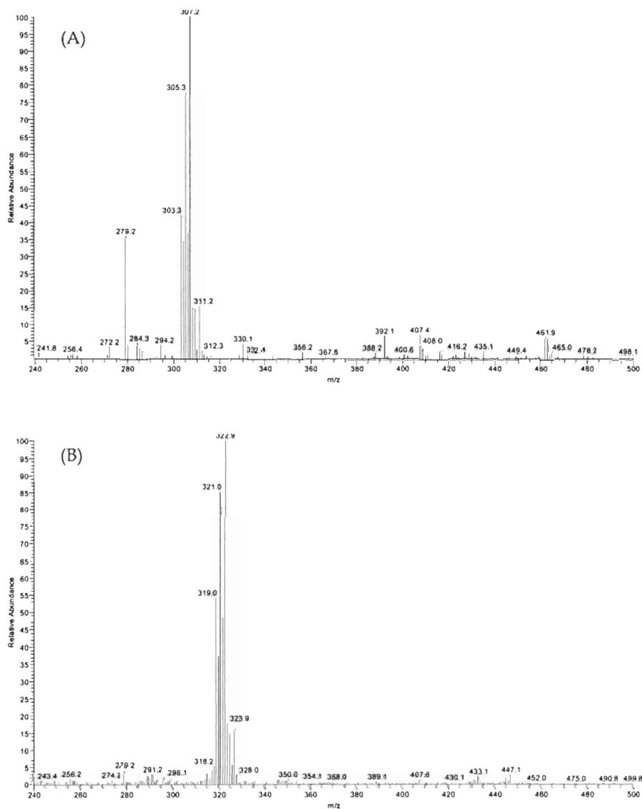
Fig. 1. Mass spectra showing the main ion group of OHBuDBT (A), TBT (B) and DBT (C, using mobile phase without tropolone and D, using tropolone in the mobile phase) acquired in the positive mode of full scan of the MS using the APCI source of the LC-MS.
