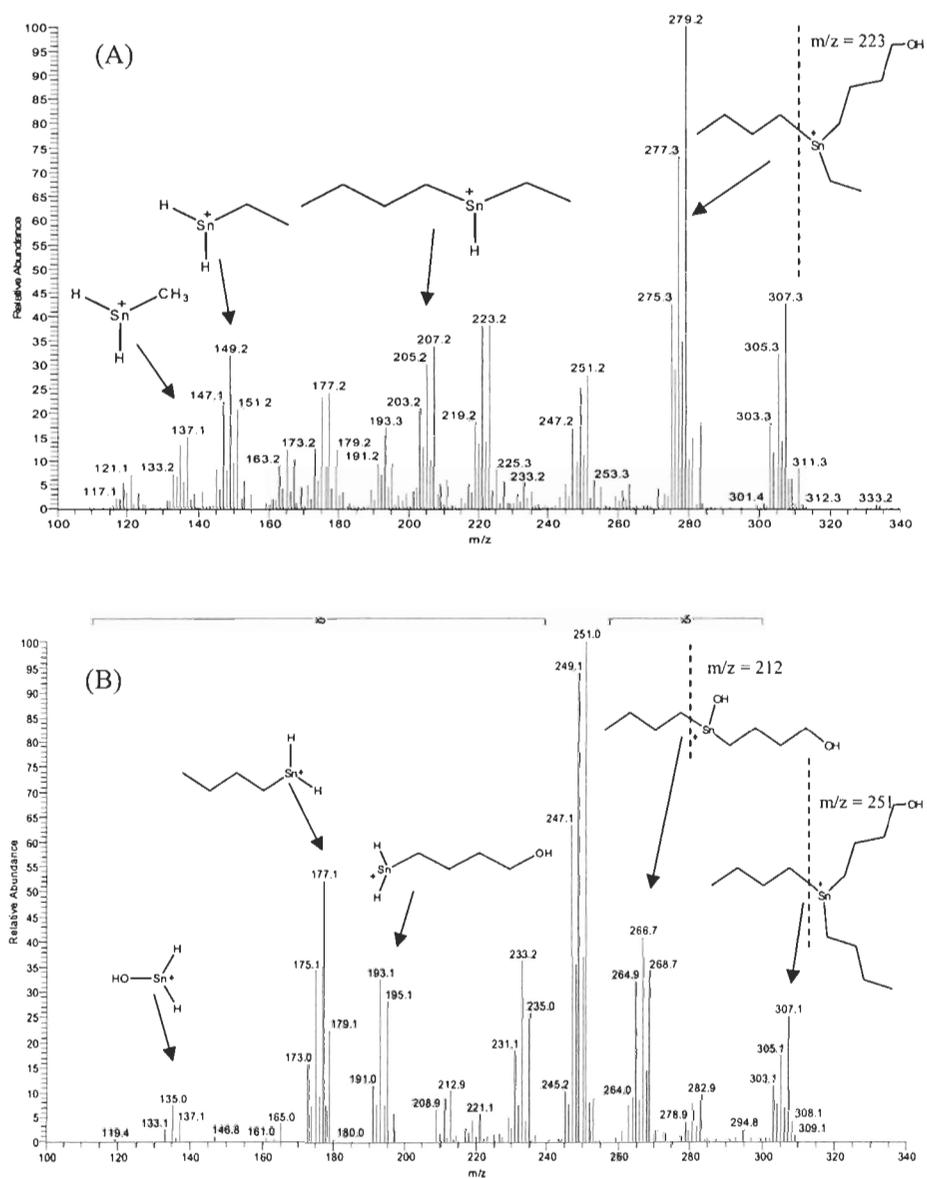
Fig. 2. GC-MS mass spectrum (A) and APCI-MS/MS spectrum (B) of 4-OHBuDBT acquired in the full scan mode.
