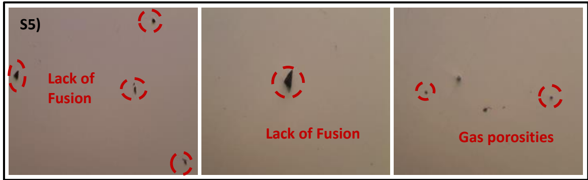
Figure 3.7: Optical micrographs showing defects in 17-4 PH stainless steel specimen S5 fabricated by LPBF and treated with H900 condition.
