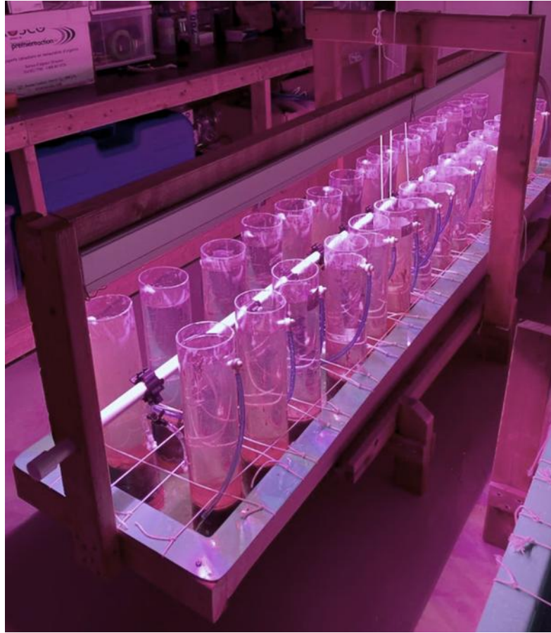
Figure S 2: Experimental setup to maintain eelgrass plants in running seawater during exposure to contaminated sediment. Copyright Cloé Falcoz.
