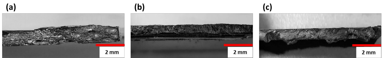
Figure 4.8 Physical appearance of fractured tensile specimens (a) AA7075/Ti6Al4V joint, (b) AA7075 BA and (c) Ti6Al4V BA
