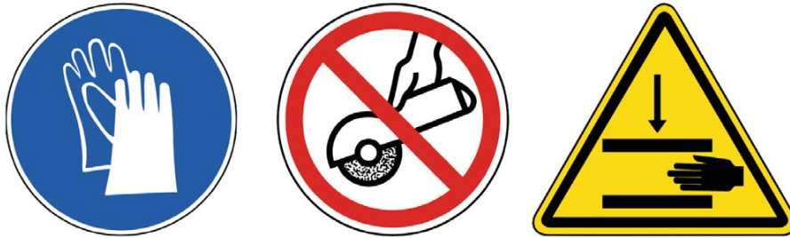
Figure 21: Examples of international safety symbols. From the left: a mandatory symbol, a prohibition symbol and a warning
