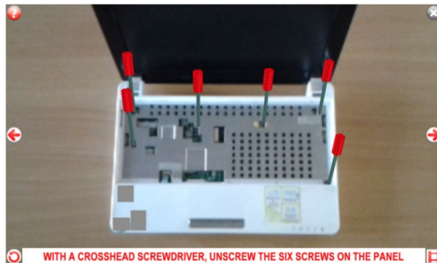
Figure 7: Step by step assembly [64]
