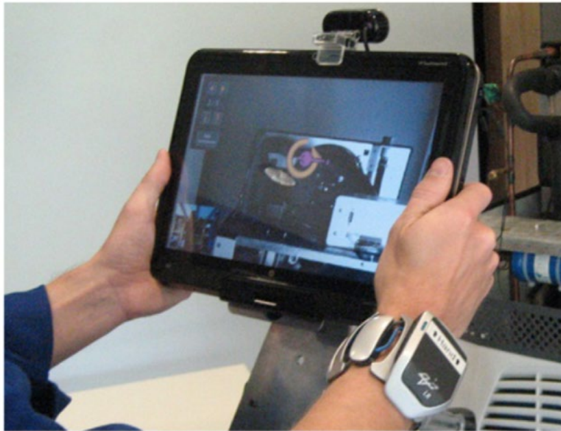
Figure 12: Example of the utilization of a vibrotactile bracelet for supporting maintenance tasks [76]
