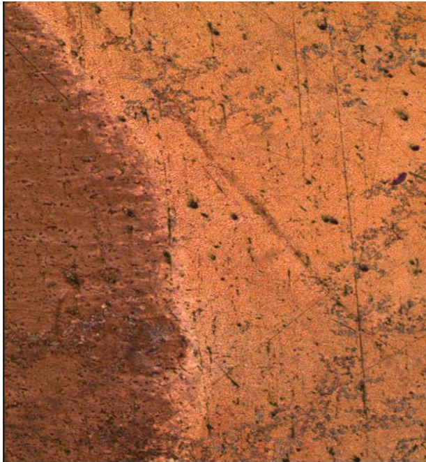
Figure 23. Microstructure at the fusion line of the sample 3
