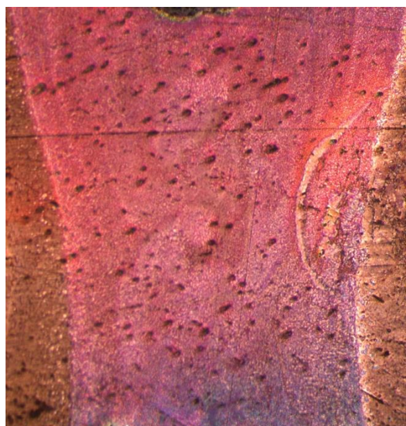
Figure 24. Microscopic holes observed in the welding pool in samples 5 and 6
