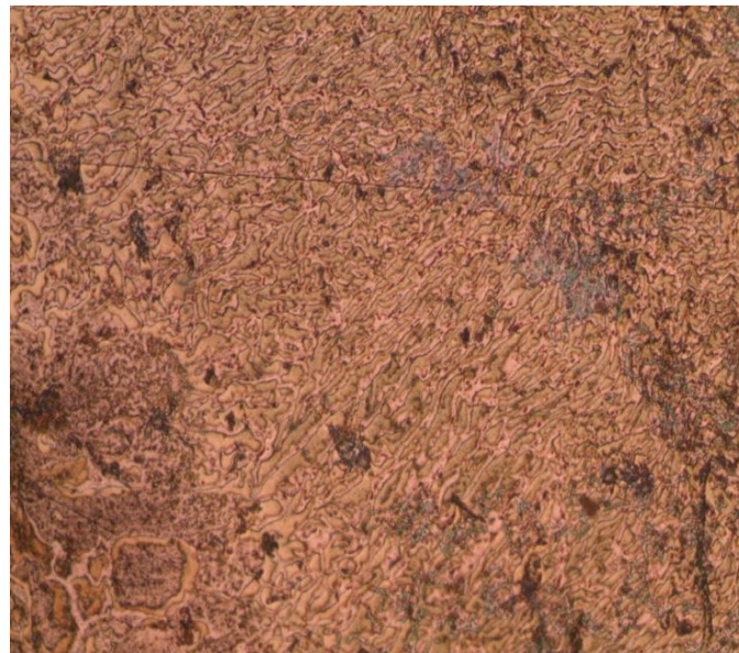
Figure 22. Dendrite observed in the base metal
