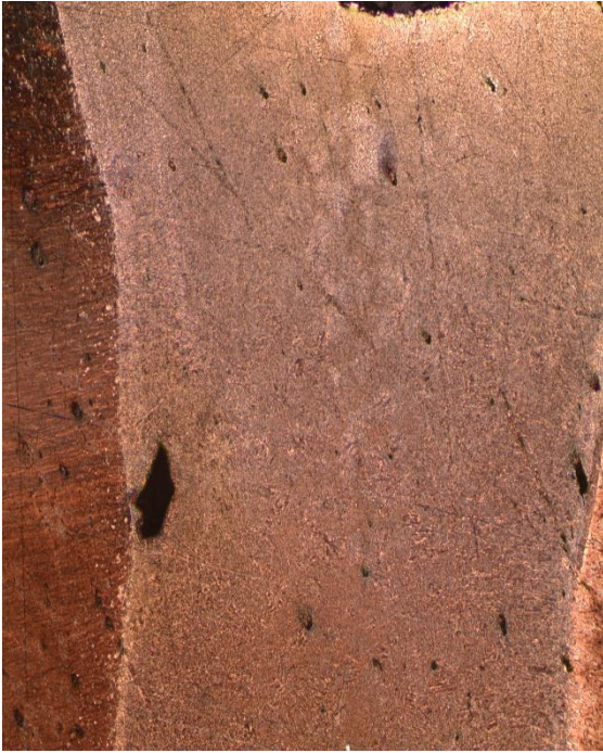
Figure 25. Formation of the porosities seen in the samples 7 and 8
