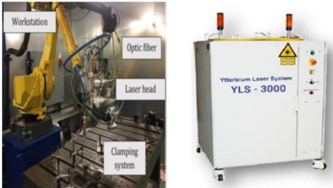
Figure 3.1 (a) Fanuc®M-710iC robot and HIGHYAG BIMO laser head (b) YLS-3000 laser source
