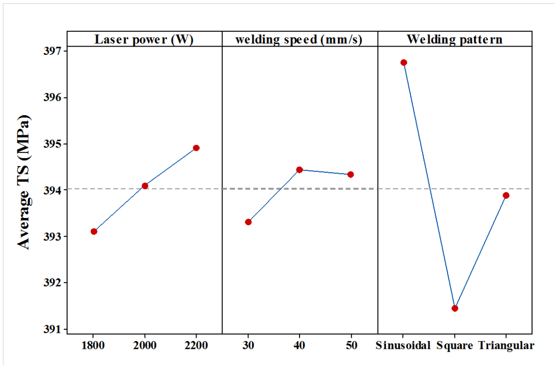
Figure 2.13 Graph of the main effects of the UTS response for A653 galvanized steel
