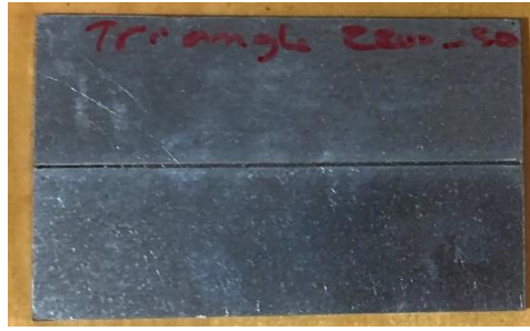
Figure 3.2 Top view of ASIS 304L sheets welded in a butt joint configuration
