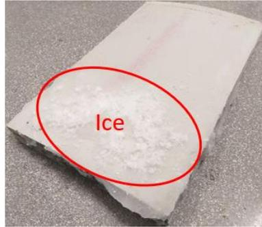
Figure 95. Ice on specimen
