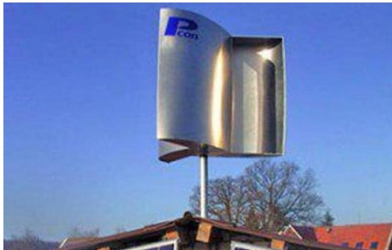
Figure 19. Savonius turbine
