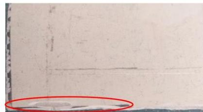
Fig. 7. Moderate erosion on the blade specimen.
