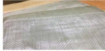
Fig. 6. Glass fiber composite samples.
