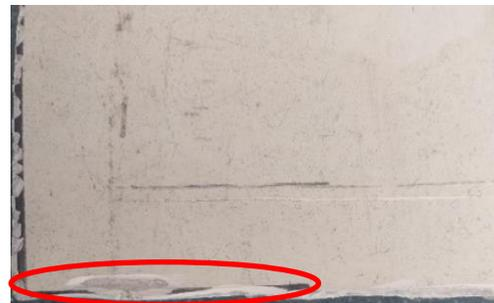
Figure 81. Severe crack on the blade specimen
