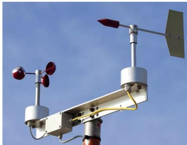
Figure 46. Anemometer and Vane [225]
