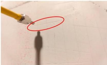
Fig. 4. Minor scratch on the blade specimen.
