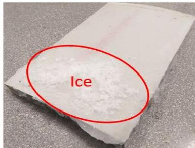
Figure 82. Ice on the specimen
