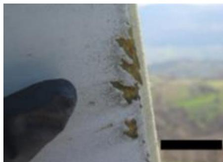
Figure 27. A small area of coating damage [131]
