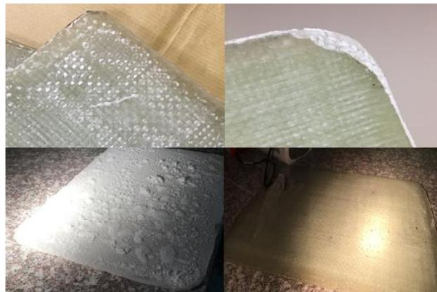
Figure 61. Faults on the tested specimen
