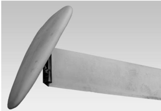
Figure 5. A tip flap aerodynamic brake
