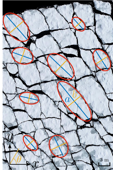
Figure 9: Sample of the ellipses fitted on the ice floes by Matlab. Blue lines indicate the major axes ( a ) and yellow ones show the minor axes ( b ).
