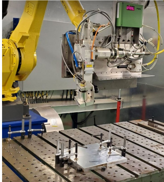
Figure 20. Automatic fiber laser system, six-axis robotic system FANUC M-710ic with IPG Photonics YLS-3000 (ytterbium fiber lasers).
