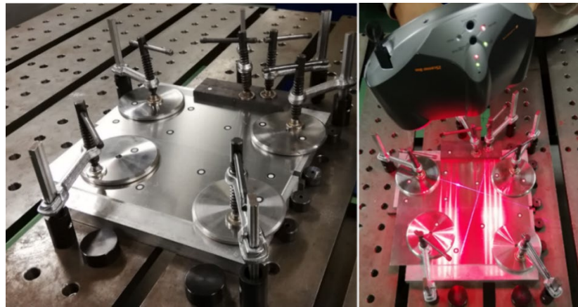
Figure 19. 3D laser scanning setup, reference points and equipment.
