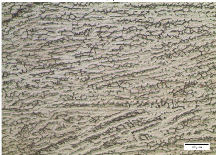
Figure 1.5 Optical micrographs of welded AISI 304L showing: (a) HAZ, (b) Fusion Line, and (c) Weld Metal.
